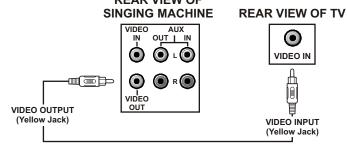
If your television does not have the required Video Input, you will need an RF Modulator (Radio Frequency Modulator), which connects through your TV Antenna or cable line and serves as Video Input.
